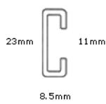
► This Top Rail is aluminium and is made in 2m lengths, dimensions as shown.
