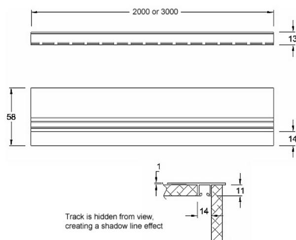
► This top rail has been designed to accommodate a sophisticated and strong picture hanging solution at the building or architectural stage. It is recessed into the ceiling, ideal where tracking needs to be hidden
